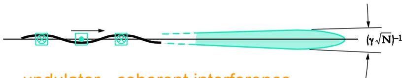
undulator - coherent interference
